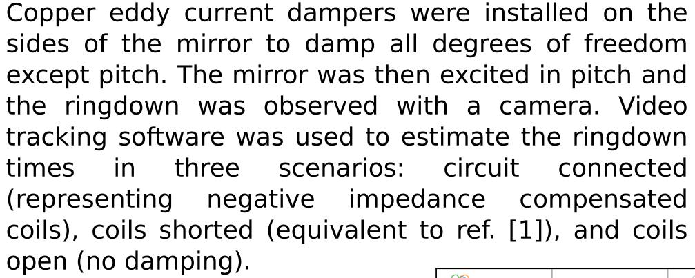
The negative impedance compensated coils are damped extremely quickly, with a time constant (1/e) of around **0.6 s**, compared to 50 s and 115 s in the case of the shorted and open coils, respectively.
