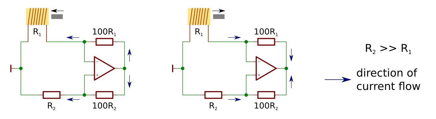
By carefully tuning the ratio of the positive and negative feedback voltage dividers, very high damping can be achieved. The division ratio of the
