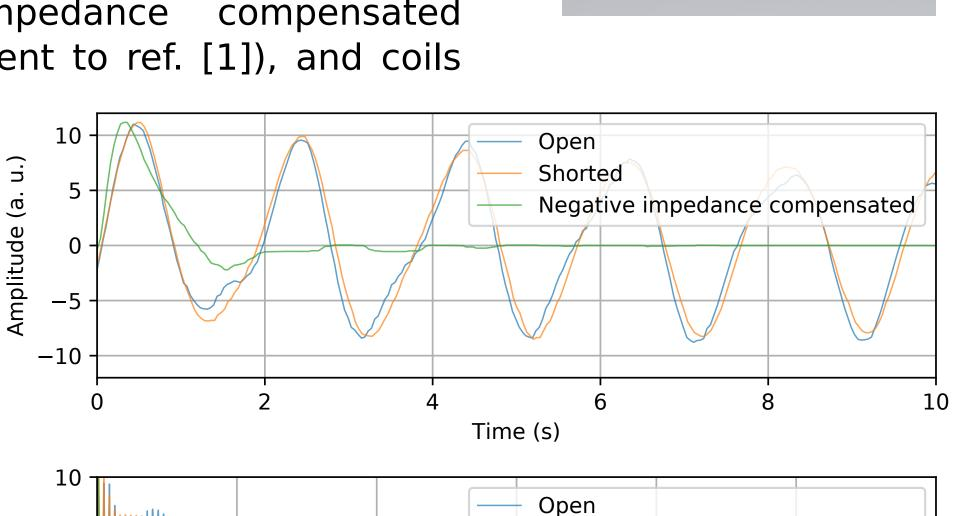
positive and negative feedback paths must be similar to achieve highest damping, with the positive path slightly lower than the negative path to avoid instability. The ratio between the resistors connecting the op-amp's output to its inputs sets the suppression. In theory, the positive feedback resistances should be much larger than the negative feedback resistances, but current and thermal noise considerations must be made when choosing values for a given op-amp.
