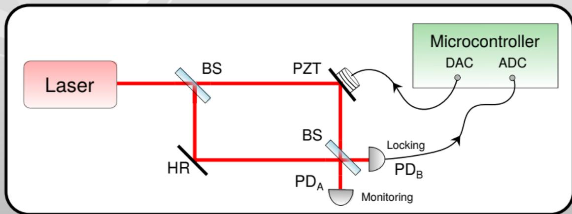
Searching algorithm is implemented in the microcontroller to lock the interferometer.
