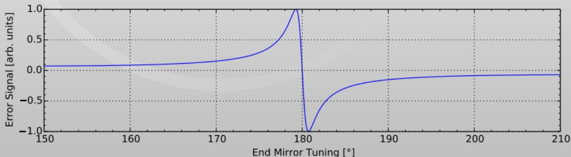
In the microcontroller, it is possible to differentiate the DC signal in order to obtain information about the cavity's direction of travel (and thus feedback a compensating impulse):
