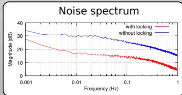
With a microcontroller, the actuator range can be re-centred before it reaches its limit. In the Mach-Zehnder experiment, this was required roughly once per hour, and allowed it to be locked for 7 hours:
