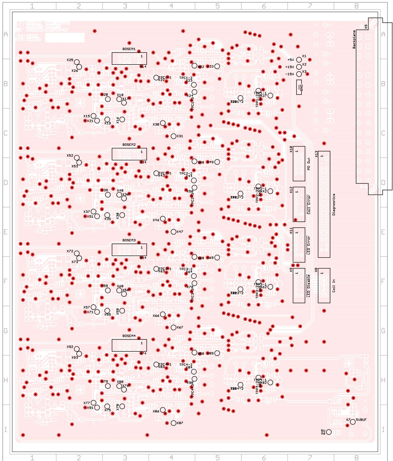
**Figure 22:** Board top view showing connectors, test points, vias and wired components
